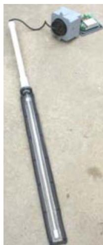
**Figure 8 – Removing the UV lamp support frame**
